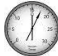
Check Ignition Timing Steady Low 15-18 Hg
