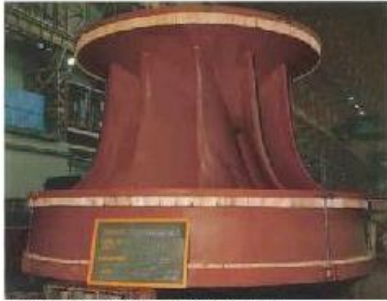
Runner for 51.4MW turbine with 41.5m head
