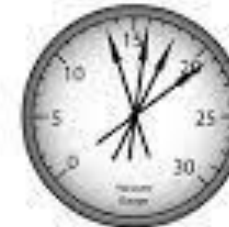
Sticking Valve or Misfire Fluctuating Needle
