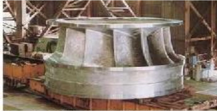
Runner for 325MW turbine with 116.2m head
