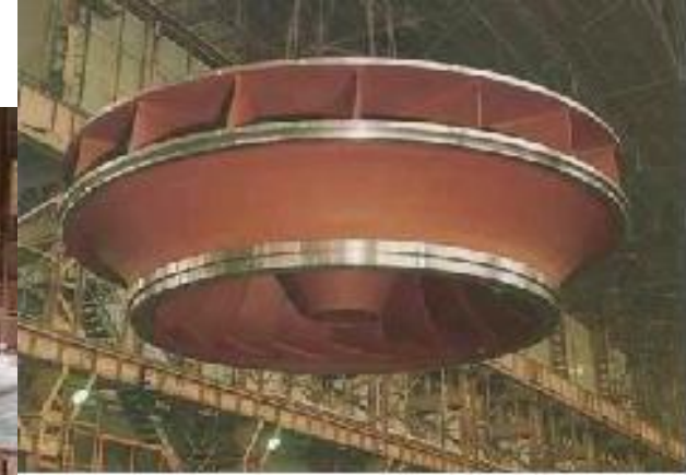
Runner for 268MW turbine with 411m head
