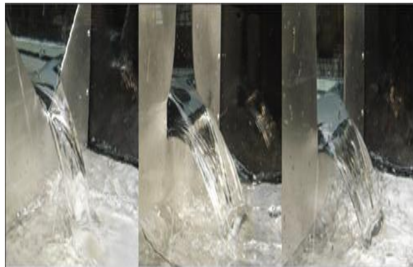
V-notch, Sutro and Rectangular plate weirs Trapezoidal and Sharp Crested weirs also included with the S6-20.
