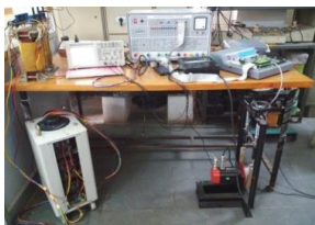
FPGA based Permanent Magnet synchronous machine control
