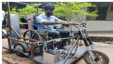
Electric Three-Wheeler with Foldable Ramp for Physically Challenged
