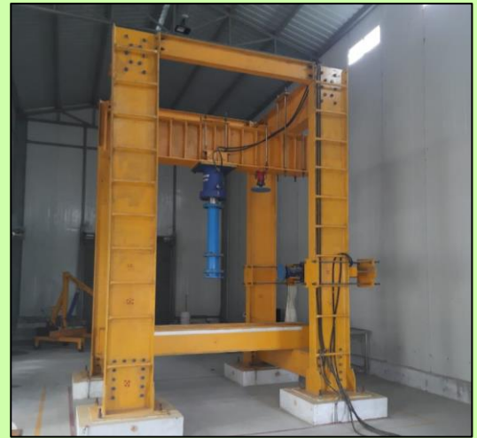
Loading Frame set-up
