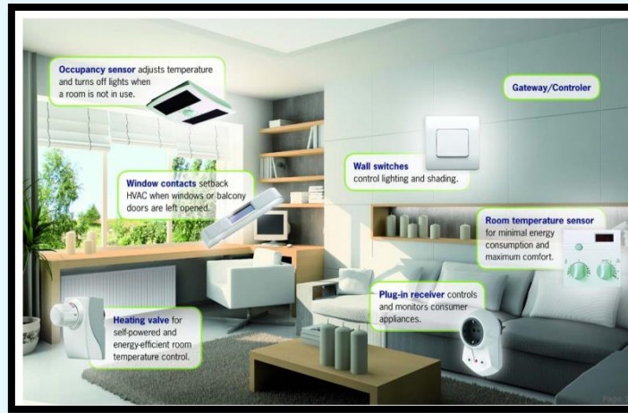
Figure 1: Wireless and Battery-less System for Smart Residential Buildings.
