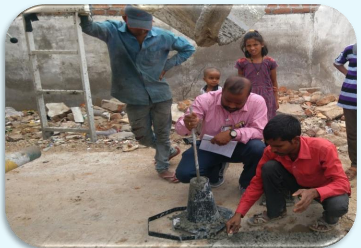
Dr. R. Durga Prasad involved in Slump testing
