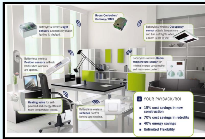
Figure 2: Wireless and Battery-less System for Smart Commercial Buildings.
