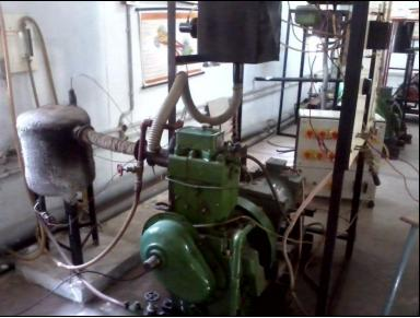
Single cylinder four stroke diesel engine test rig
