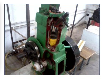
Cut Model of Diesel engine
