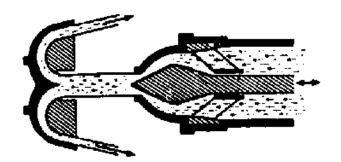
Fig. 9: Jet Impinging on Bucket
