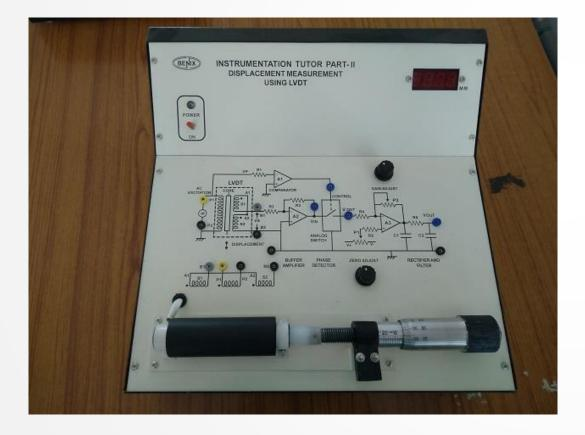
**LVDT** is an acronym for Linear Variable Differential Transformer. It is a common type of electromechanical transducer that can convert the rectilinear motion of an object to which it is coupled mechanically into a corresponding electrical signal.
