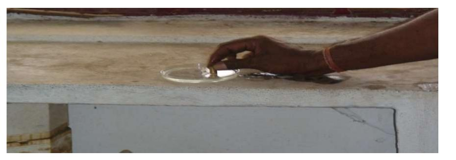
• Clean the specimen with cotton waste after etching
