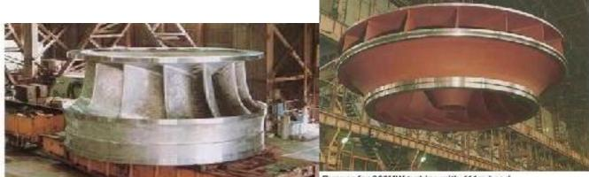
Runner for 266MW turbine with 411m head
