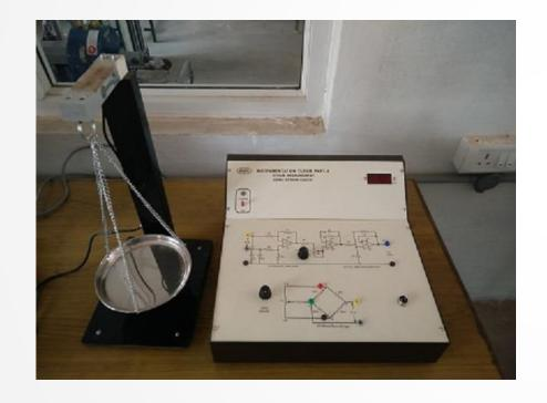
A load cell is a force transducer. It converts a force such as tension, compression, pressure, or torque into an electrical signal that can be measured and standardized. As the force applied to the load cell increases, the electrical signal changes proportionally.
