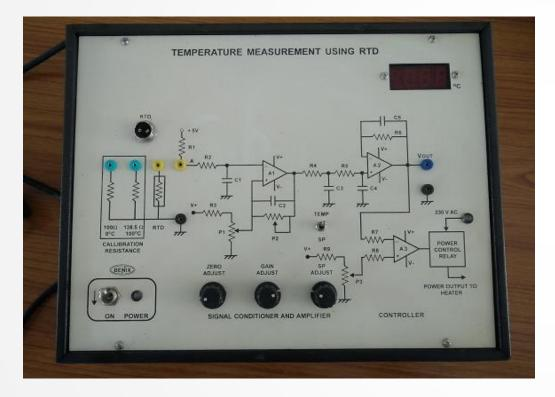
**Resistance thermometers**, also called **resistance temperature detectors** (**RTDs**), are sensors used to measure temperature. The RTD wire is a pure material, typically platinum, nickel, or copper. The material has an accurate resistance/temperature relationship which is used to provide an indication of temperature.
