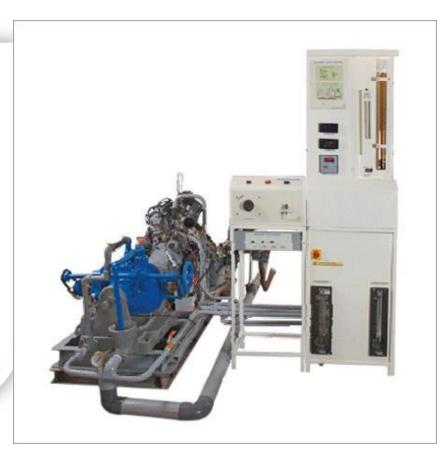
Computatised single cylinder four stroke diesel engine test rig
