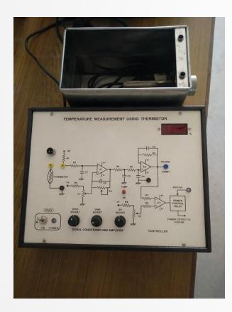
A **thermistor** is a resistance thermometer, or a resistor whose resistance is dependent on temperature. The term is a combination of "thermal" and "resistor". It is made of metallic oxides, pressed into a bead, disk, or cylindrical shape and then encapsulated with an impermeable material such as epoxy or glass.
