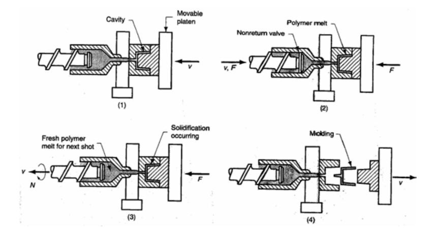
Cycle of operation for injection molding
