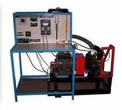
Single cylinder four stroke petrol engine test rig
