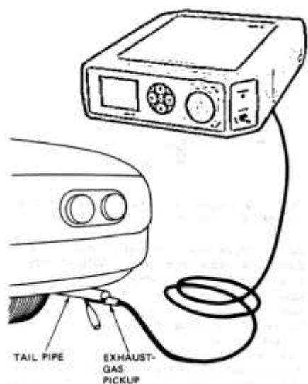
Figure 3: Five-gas analyzer connected to tailpipe of a vehicle to test the exhaust gas
