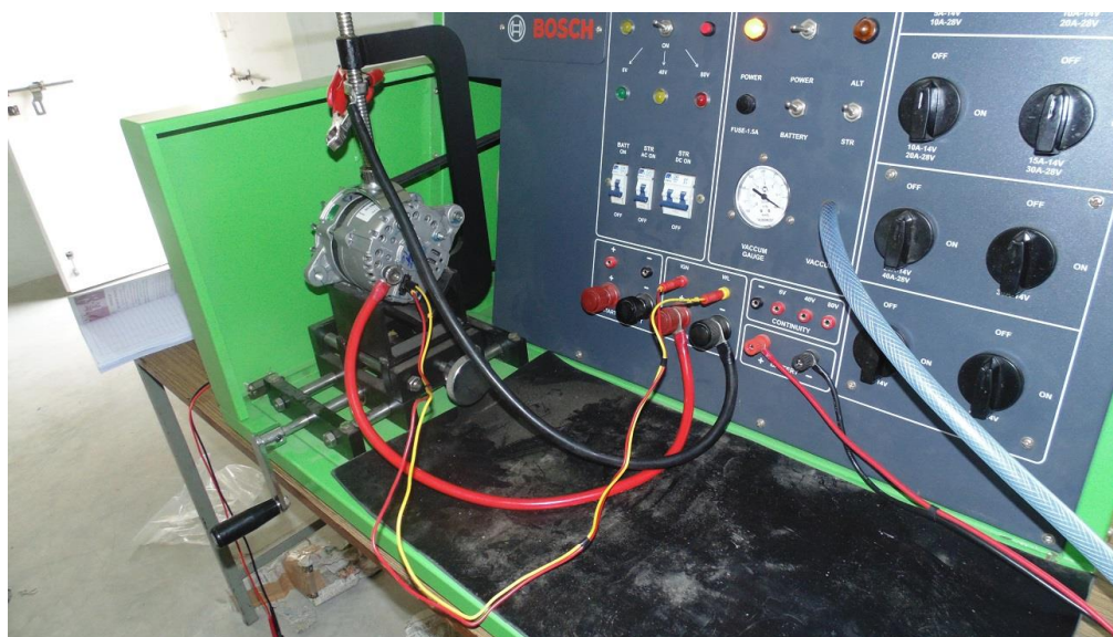
Fig 6. Alternator Test Set-up
