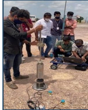
Field Testing of LWD designed and developed apparatus
