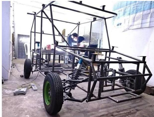
The chief objective is to create a strong and well balanced skeleton for the vehicle to provide proper support structure and a rigid means for all the other mountings on the vehicle. The chassis has been designed using highly durable and considerably light, AISI 4130 steel suitable to absorb all the real-time impacts and roll over loads.
