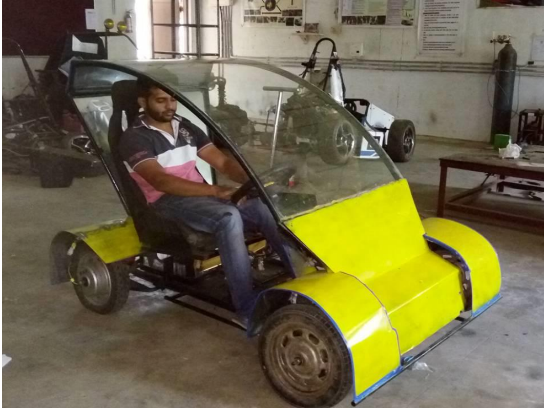
Electric Micro-car with hub motors as part of center of Excellence
